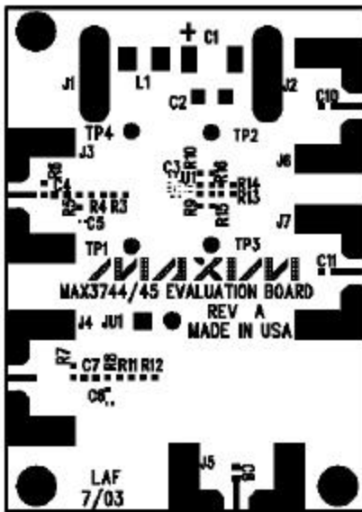
Figure 2. MAX3744/MAX3745 EV Kit PC Component Placement Guide—Component Side
